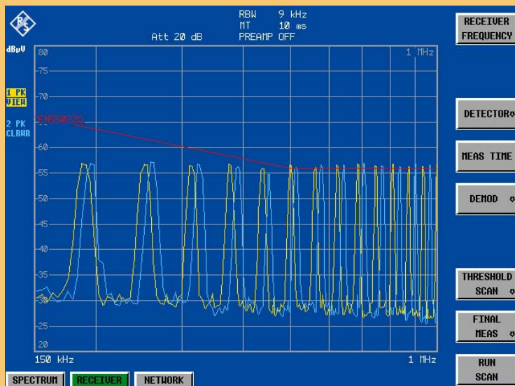
FIG 1 Two cycles recorded several minutes apart. The interference signal, measured with the V-Network R&S®ENV 216 on a switching power supply, has clearly left the measurement bandwidth.
