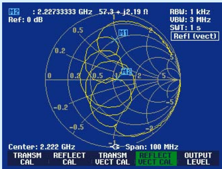
FIG 2 Vector reflection measurement of a multicircuit bandpass filter.
