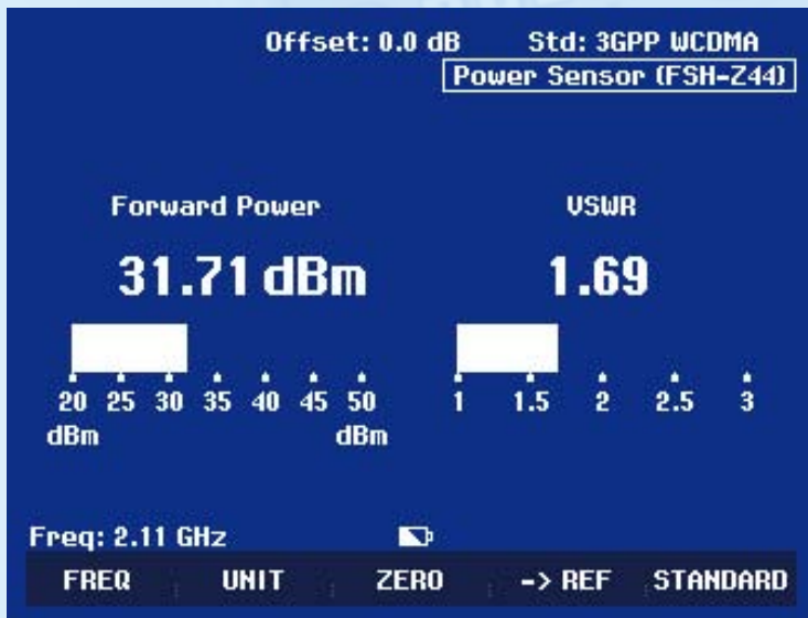
FIG 5 Simultaneous display of the transmitter output power and the antenna matching.
