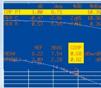
FIG 4 Zoom view of FIG 3 – compression point (1 dB), reduction of mean power and of crest factor at current modulation of DUT.
